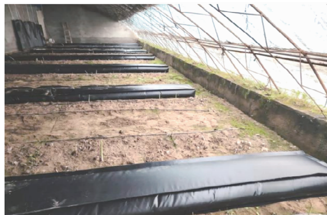
Fig. 1 Actual heat storage water bags inside the greenhouse
